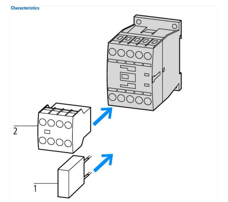
1: Suppressor 2: Auxiliary contact module
