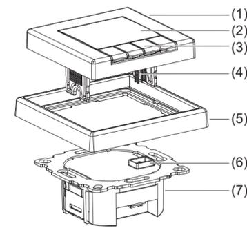
Fig. 1: Layout of the temperature controller
