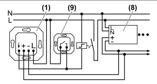
Figure 5: Connection diagram for potentiometer with push-button function and extension
