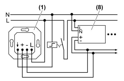
Figure 4: Connection diagram for potentiometer with push-button function
