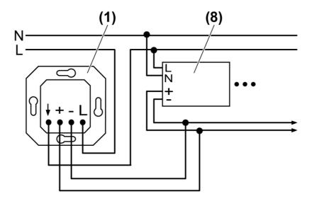
Figure 2: Connection diagram for potentiometer with switching function
