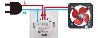
4.2 Control the appliance lower than 500W (Eg:1CH).
