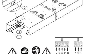
Next, slide the other luminaire onto the other ends of joining kit and tighten the screws. Connect the plugs or through-wiring together and connect one of the fittings to the power accordingly to the markings on the connection terminal and the drawing above.
