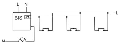
Relay version "i" is to pin adapted to cooperate with the receivers with high starting current, such as LED fluorescent lamps, ESL fluorescent lamps, electronic transformers, discharge lamps, etc.
